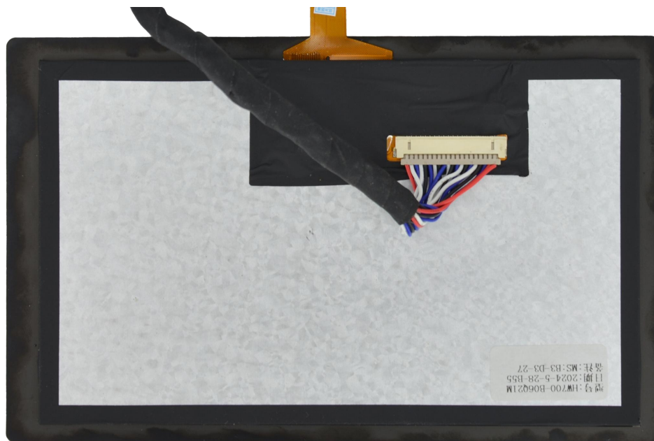
Figure 25 Connect LVDS screen cable to DEBIX Model C
