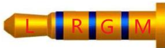
Figure 15 Definition of four-segment headphones
