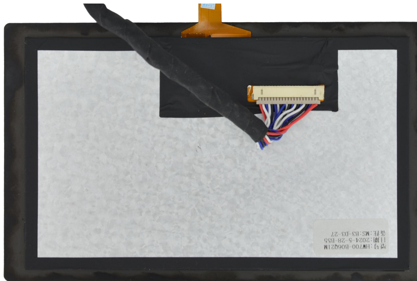
Figure 26 Connect LVDS screen cable to LVDS screen
