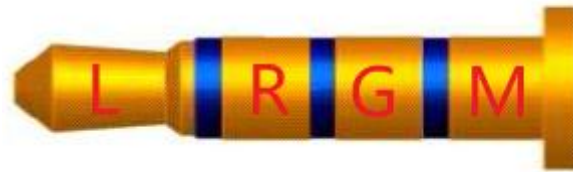
Figure 32 Definition of four-segment headphones
