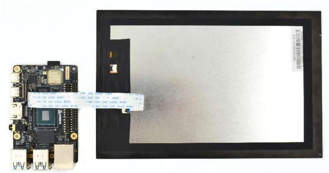
Figure 63 MIPI screen to DEBIX completed
