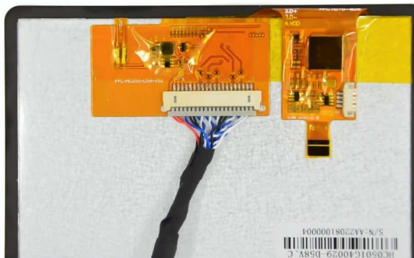
Figure 67 Connect LVDS screen cable to LVDS screen
