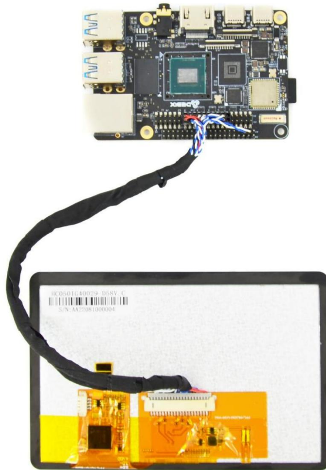
Figure 68 LVDS screen to DEBIX completed
