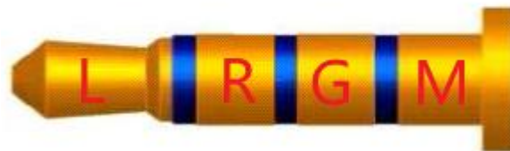
Figure 18 Definition of four-segment headphones
