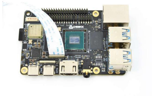
Figure 62 Connect FPC cable to DEBIX
