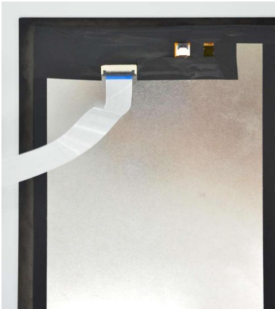
Figure 61 Connect FPC cable to MIPI screen
