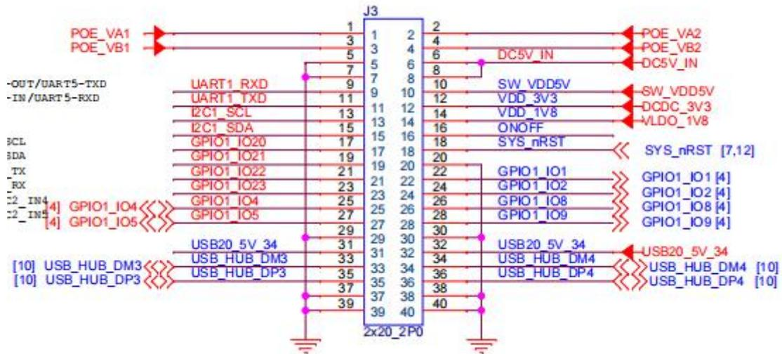
Figure 17 Pin sequence of GPIO
