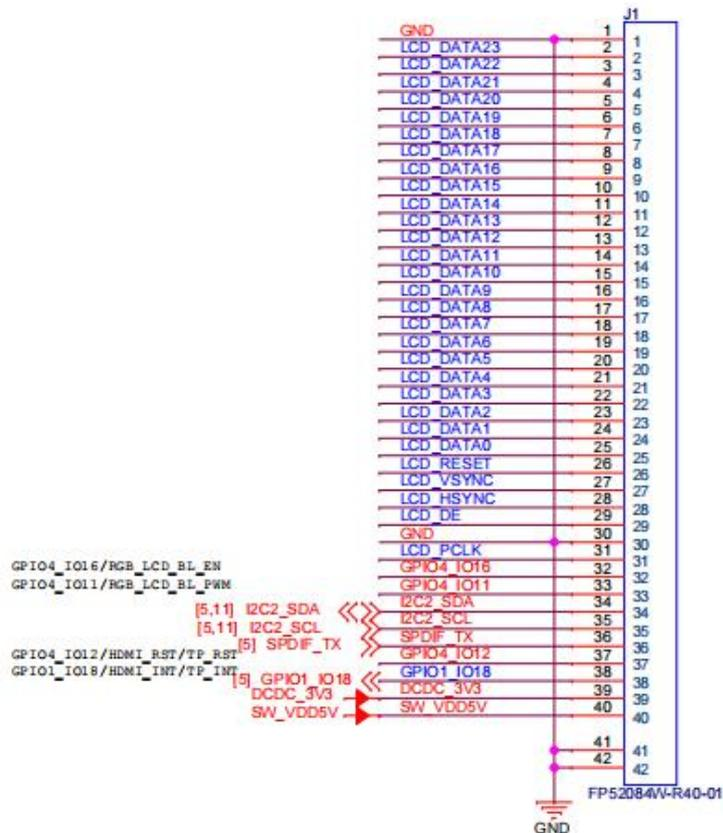
Figure 11 Pin sequence of RGB
