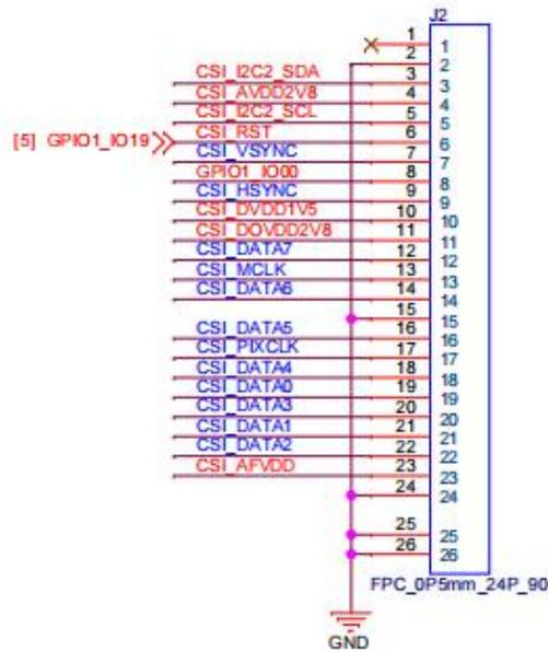
Figure 13 Pin sequence of CSI
