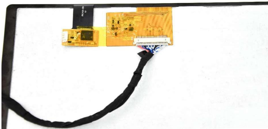
Figure 72 Connect LVDS screen cable to LVDS screen
