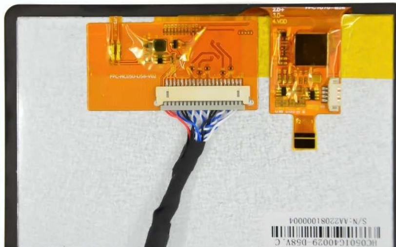
Figure 67 Connect LVDS screen cable to LVDS screen
